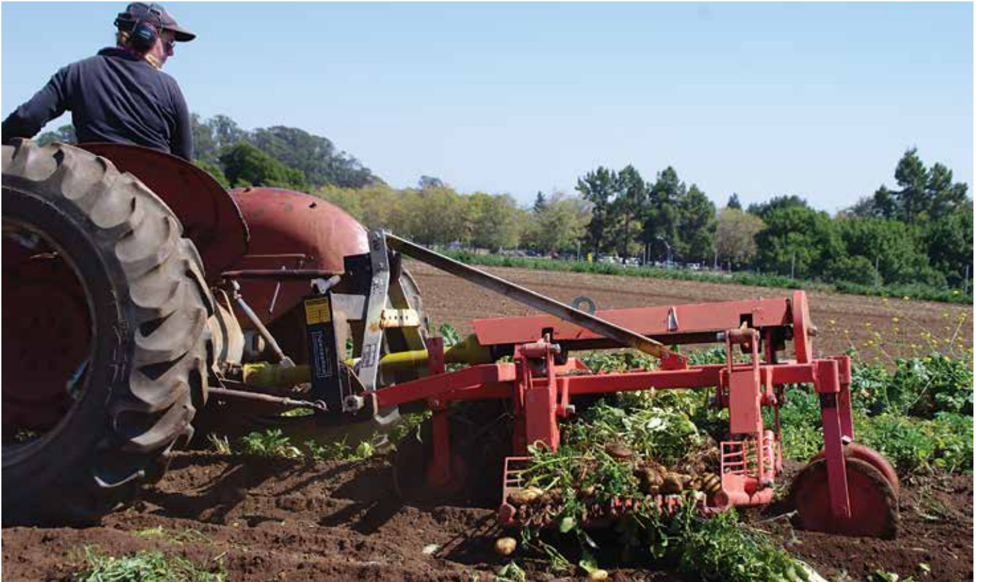
FIGURE 9. Example of a PTO-driven harvester with “shaker cage.” Photo: Martha Brown
